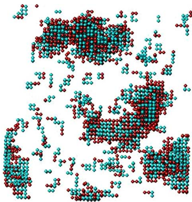
Fig. 4 Final configuration of the box of simulation. As is clear at volume fraction of 0.04 of H_2T_4 , some aggregates have cylindrical shapes
